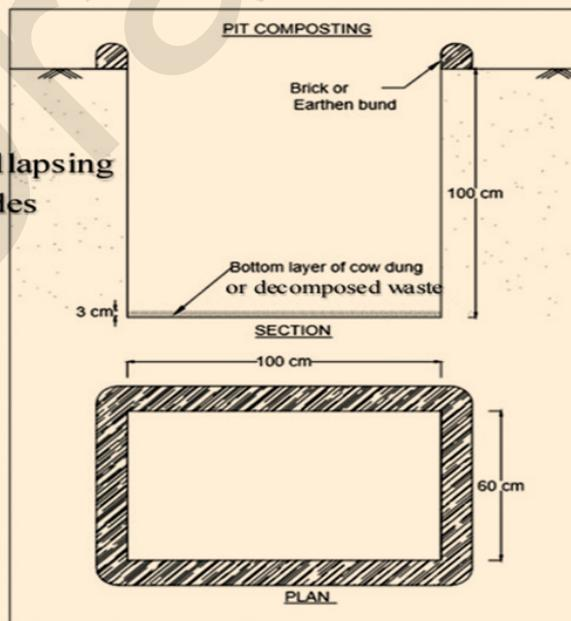
*Section and Plan of Pit for Composting*
